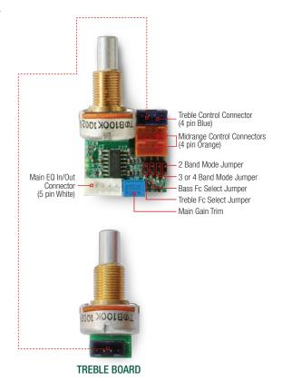
The Midrange Boards are functionally identical except for the parts that determine the frequencies they control. You can use either one or both interchangeably.
