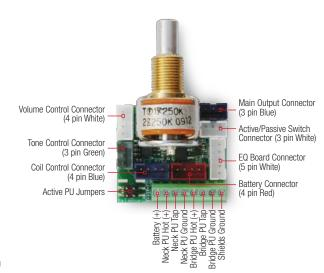
**EQ Board Connector** – Connect this , through the supplied 5 pin wire harness, to the White 5 pin connector on the EQ Board.
