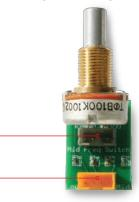
The Balancer Board is where all the signals get in and out of the preamp. Depending on the configuration of your preamp, this board may have a balancer or a single Neck Pickup Volume control on it. The pickups connect straight to the screw terminals. Simply strip the wires and insert them into the appropriate terminal. Then tighten the screw down tight. There will be more detailed instructions on connecting pickups later in this manual.
